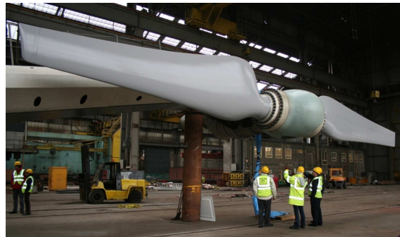
Figure 5.7 – Carbon fibre rotor blades for the 'SeaGen' tidal current turbine. (Courtesy of Marine Current Turbines Ltd: http://www.marineturbines.com/ ).
