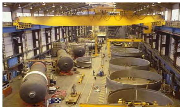
Figure 3.14 – Steam Generator fabrication at Mitsui (now Doosan) Babcock, Renfrew, for Sizewell B. (Courtesy of Doosan Babcock Energy Ltd.)
