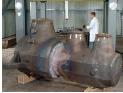
Figure 2.7 - Main stop valve body for a super-critical application, produced from two 10Cr-MoVWNbN, P911 castings, weld fabricated to make a 16,000kg valve body. (Courtesy Goodwin Steel Castings Ltd.).
