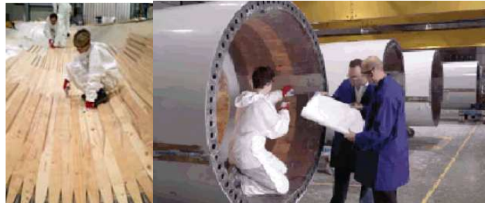
Figure 4.11 - Wind rotor blade fabrication at the Vestas Isle of Wight site.
