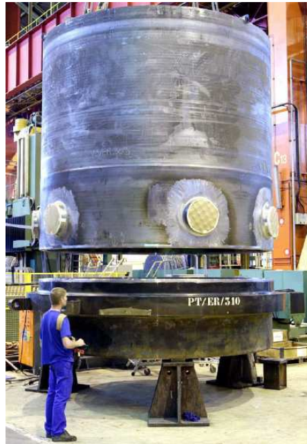
Figure 3.11 - Large Reactor Pressure Vessel (RPV) forging with nozzles. (Courtesy of Areva NP).
