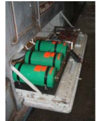
Supercap Field Trial Used for starting 1000shp diesel locomotive with Supercap provides 1500A at 60V ( courtesy of MASTCarbon Technology Ltd)
