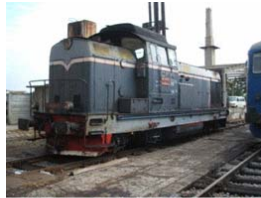
Supercap Field Trial Used for starting 1000shp diesel locomotive with Supercap provides 1500A at 60V ( courtesy of MASTCarbon Technology Ltd)
