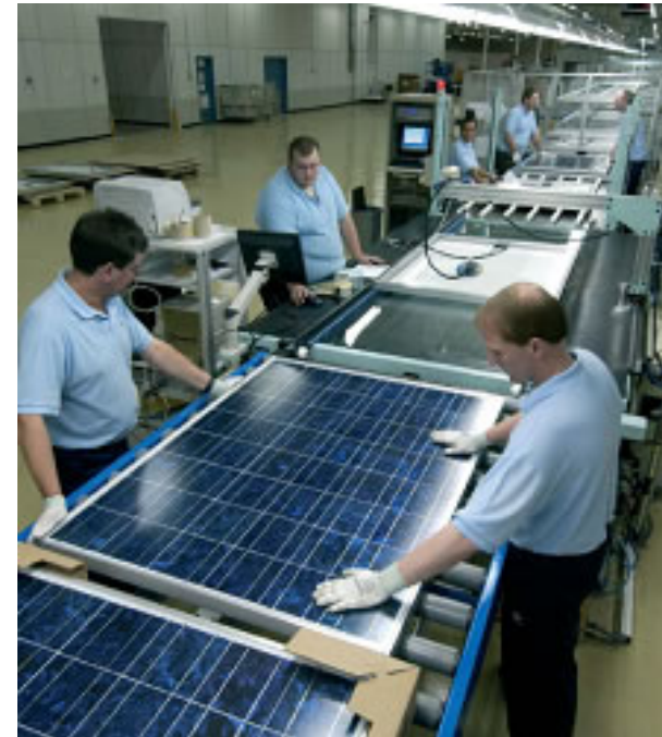
Sharp module factory near Wrexham producing 220 MW/year
