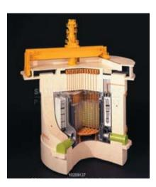
Figure 3.3 - Schematic of the Oldbury Magnox reactor, commissioned in 1968. (Courtesy of 'The Science & Society Picture Library': http://www.scienceandsociety.co.uk/)
