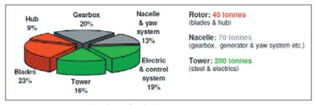
Figure 4.8 – Approximate weights and costs of wind turbine components. (Courtesy of BVG Associates Ltd.).
