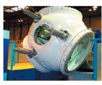
Figure 4.10 – A wind turbine nacelle bedplate casting. (Courtesy of 'WindSupply': http://www.windsupply.co.uk/).
