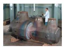
Figure 2.7 - Main stop valve body for a super-critical application, produced from two 10Cr-MoVWNbN, P911 castings, weld fabricated to make a 16,000kg valve body. (Courtesy Goodwin Steel Castings Ltd.).
