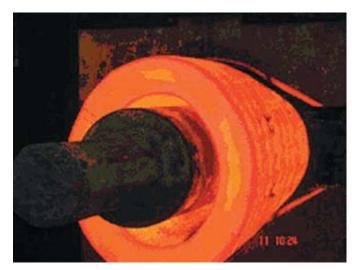
Figure 3.10 - Large Reactor Pressure Vessel (RPV) forging. (Courtesy of Areva NP).
