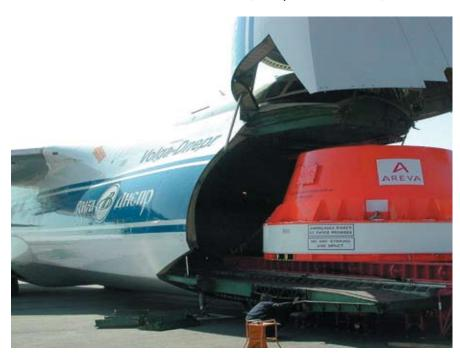
In 2006, the head of the Sizewell B reactor was replaced. The replacement head was manufactured by Areva and was the same as the original head (ASME SA 508 Class 3, low alloy Mn-Mo-Ni steel), but because of stress corrosion concerns, used Inconel 690 welds between the head and control rod guide tubes, instead of the Inconel 600 welds, which were used on the original head. The proposed investment at Sheffield Forgemasters would give a UK-based RPV Head forging capability.
