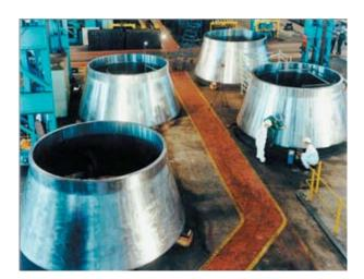
Figure 3.16 - Steam Generator transition cones. (Courtesy of Sheffield Forgemasters International Ltd.).
