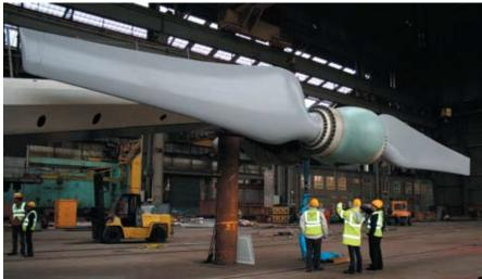
W. Berks). The rotors allow variable pitch to optimise efficiency, irrespective of tidal flow direction.
