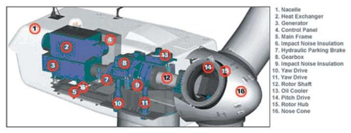
Figure 4.7 - Major components of a wind turbine (from the Scottish Enterprise document: 'Doing Business with the Wind Turbine Manufacturers: Becoming Part of Their Supply Chain', July 2006). (Courtesy of Scottish Enterprise: http://www.scottish-enterprise.com/).
