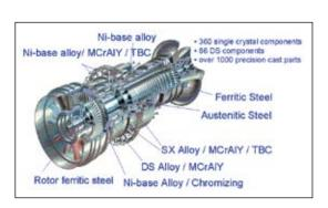
Figure 2.6 – Schematic of a gas turbine engine annotated with some of the materials of construction. (Courtesy of Alstom Power Ltd.).
