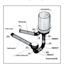
Both the high integrity pipework and the more conventional pipework is similar to that found in fossil-fired power plants and chemical plant, for example, and is manufactured from drawn pipe and cast or forged components (elbows, tees, end caps, etc.) in austenitic stainless and ferritic steels.
