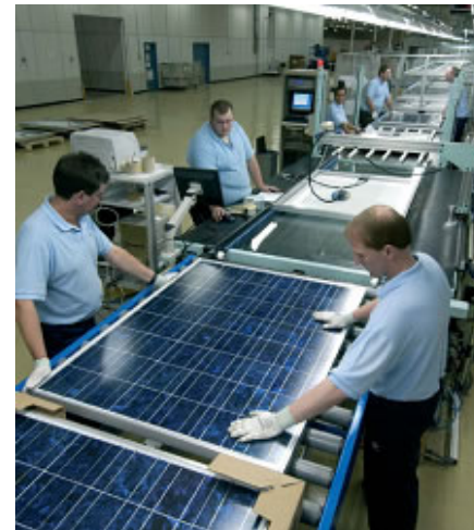
Sharp module factory, Wrexham Manufacturing 220 MW per year for the European market.
