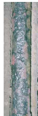
Corrosion of superheater materials in a Swedish biomass plant
