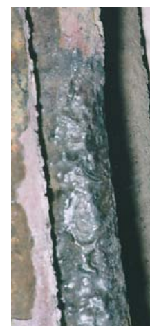
Corrosion of superheater materials in a Swedish biomass plant
