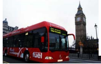
PEM Fuel Cell powered bus
